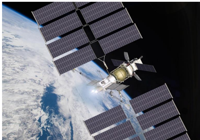
Concept of a 300 kW VASIMR ® -SEP space tug with attached payload
