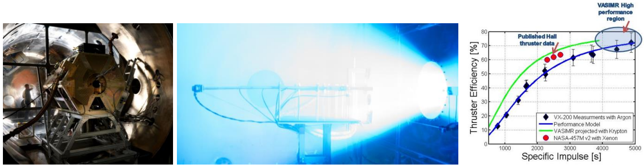
VX-200 engine (left), 200 kW argon plume (center) and measured and predicted performance data for Argon and Krypton
