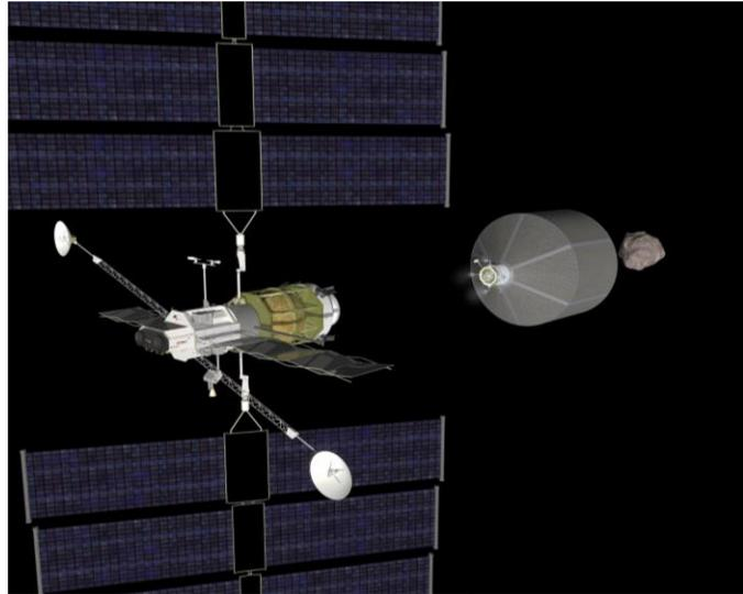
Figure 1: Concept of a 200 kW VASIMR<sup>®</sup> engine adapted to KISS study NEA retrieval module
