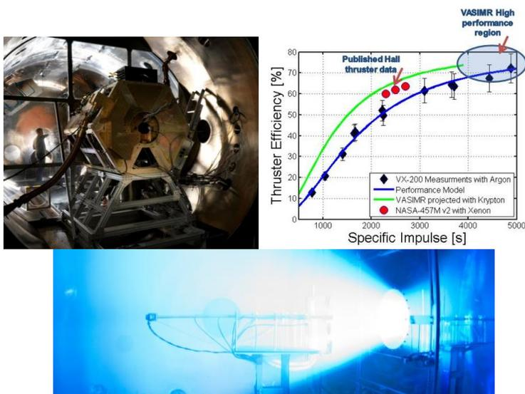
Figure 3: 2011 VX-200 performance data, VX-200 engine, and VX-200 plume at 200 kW
