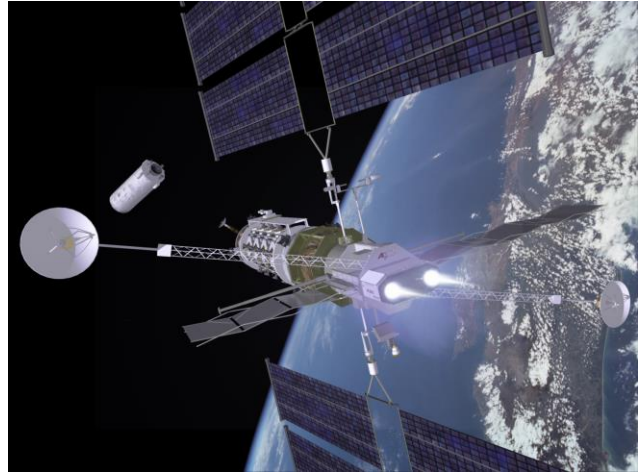
Figure 1: Powered by a 200 kW VASIMR® engine, Ad Astra's solar electric LEO Space Cleaner approaches a spent Zenit upper stage for capture and disposal
